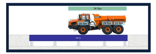
Engineered to exceed expectations, the WB-UL features a standard 24m length combined with an impressive 4.5m width. Its exceptional deck strength is built to handle total loads of up to 120T, with individual axle capacities of 50T, making it the ultimate solution for robust and reliable heavy-duty weighing.
